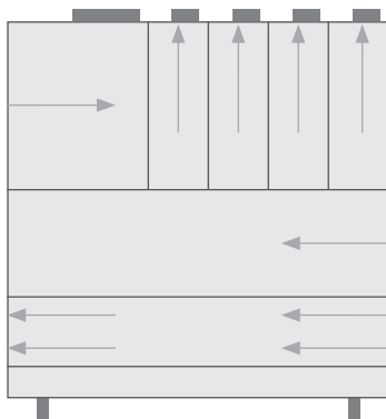
Figure 5. Top View of a Modular Power Supply With Airflow Direction Indicated
