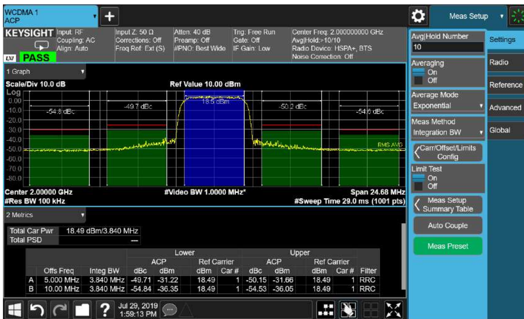
Figure 8. ACP measurement with Keysight CXA signal analyzer
