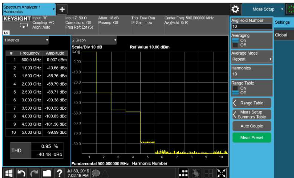
Figure 4. Harmonics measurement with Keysight CXA signal analyzer
