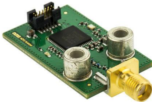
Figure 3: Analog Devices ADIS16000 Digital MEMs Vibration Sensor and RF Transceiver with Molex Brass SMA RF Connector. (Source: Analog Devices)
