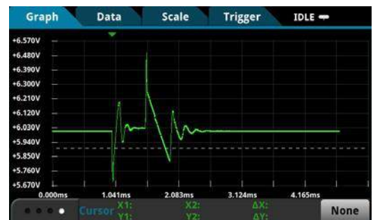
Poor response to a large load change
