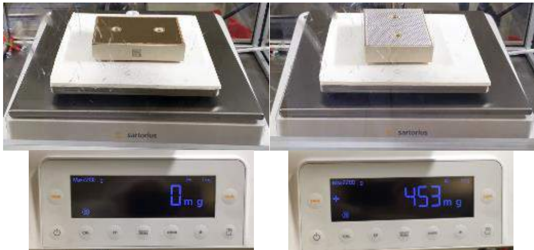
Figure 23: Measurement of module weight before (L) and after (R) paste application
