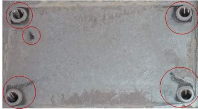
Figure 29: Black marks on heatsink resulting from heavy thermal cycling
