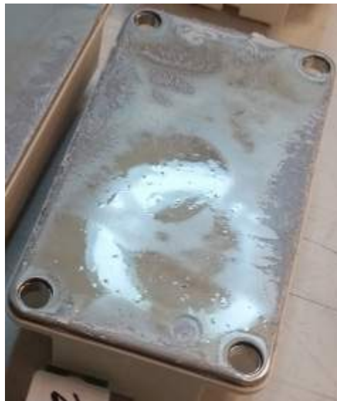
Figure 28: Underside of SEMITRANS module showing separation of carrier oil and filler after high temperature operation in the field
