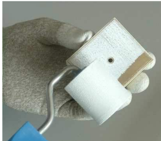
Figure 7: Applying paste to a MiniSKiiP module
