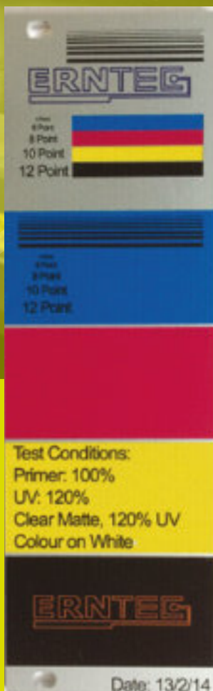
Example of a front panel printed for colour management testing
