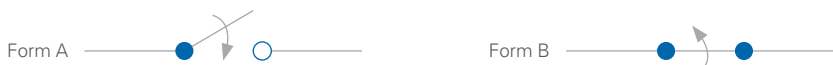
Figure 7. SPST relays come in two forms: normally open (Form A) and normally closed (Form B).
