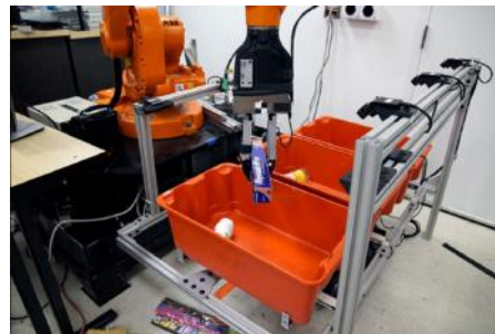
Figure 3: This robotic arm uses a vision-driven grasping algorithm to navigate gripping items of various sizes, shapes, and firmness. (Source: MIT)
