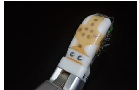
Figure 4: The “skin” in the fingertips of this hand uses a sophisticated network of fluid-filled, hair-thin channels to measure grip pressure. (Source: UCLA Engineering)
