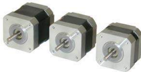
Figure 7: The HT17-268D stepper motor from Applied Motion Products is a representative unit with an industry-standard NEMA 17 frame and mounting holes. Key specifications include 1.8° step angle, 1.34 A/pole current, 31.2 oz-in minimum holding torque and 5.38 oz-in 2 rotor inertia. (Source: Mouser Electronics )
