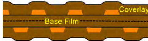
Figure 4.8 Staggered adjacent-layer traces are preferred
