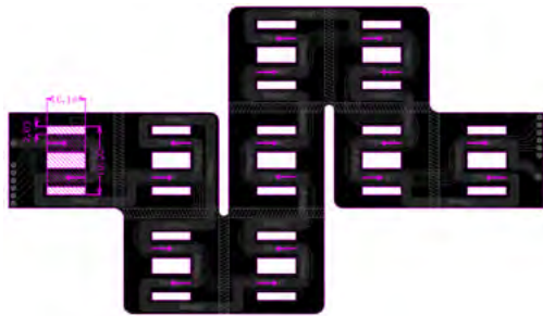
Figure 5.8 Mechanical 1 layer showing the board outline as well as winding direction arrows for guidance
