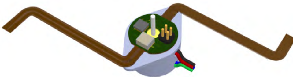
Figure 5.3 3D View of the Rotating Stepper Control Board. Longer "arms" would allow greater than 360° rotation of the motor and its control board
