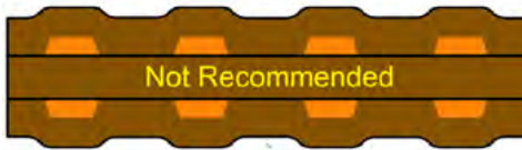
Figure 4.7 Adjacent-layer copper traces are not recommended
