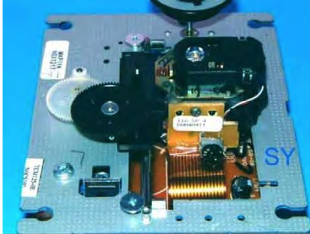
Figure 1.3 Flex-circuit used to link the laser pickup to the main board assembly in a Blu-Ray mechanism. Notice that the PCB on the laser head has the flexible portion bent at right angles, and an adhesive bead has been added for strengthening the flex circuit at the join (source: Zhuhai Smartech Electronics & Machinery).
