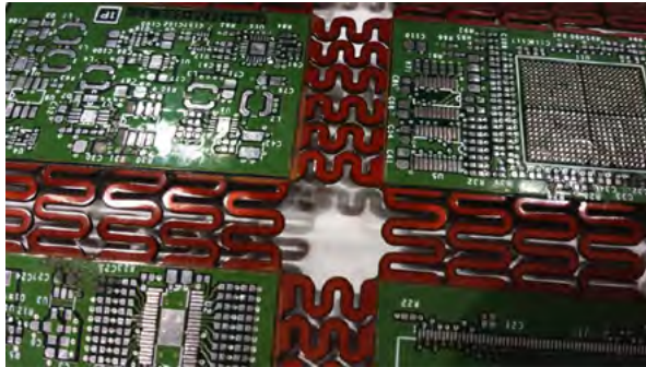
Figure 6.7 8 Layers of flex, plus 4 additional rigid layers. Notice the top layer of flex is entirely copper pour for shielding. Notice also the protective adhesive around the edges of the rigid-to-flex interfaces. (Photo: Ben Jordan)
