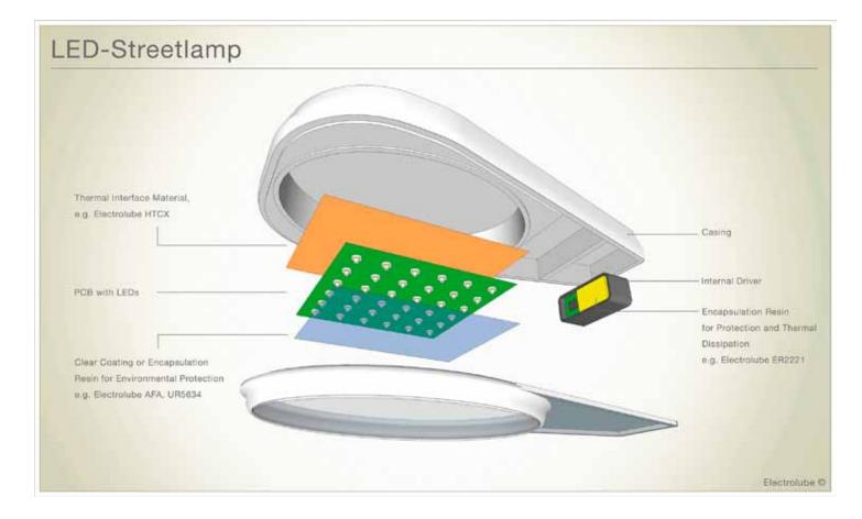
humidity or salt mist a thin layer acrylic conformal coating would offer a high level of protection with minimal impact on the light output and colour temperature of the LED. Encapsulation resins are used for harsh environments such as immersion in water, or where light dissipation and environmental protection are required in one process; Electrolube UR5635 is a good example of such a resin.
