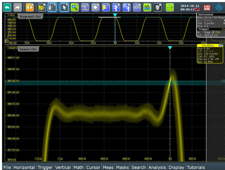
Fig. 6: The high sensitivity of the Rohde & Schwarz digital trigger makes it possible to trigger on signal overshoots of less than 9 mV, as can be seen in this example. At a vertical scale of 130 mV/div, this corresponds to only a fraction of one display division.
